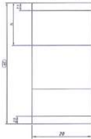
Top clamp (clamp width = 20 [mm])
