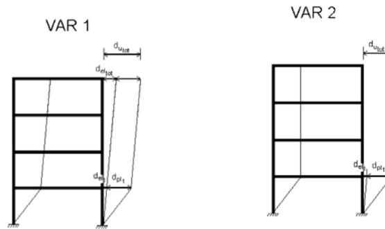
Figure 8 Structural ductility factors (left, VAR1); (right, VAR2)
