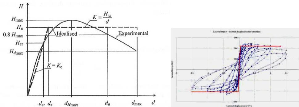
Figure 7 Bilinearization of the envelope of hysteresis
