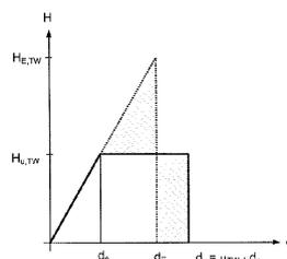
Figure 9 Structural behaviour factors
